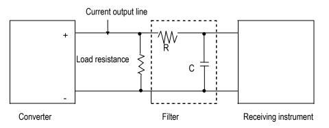
Figure 11.3 Example of Filter Connection
